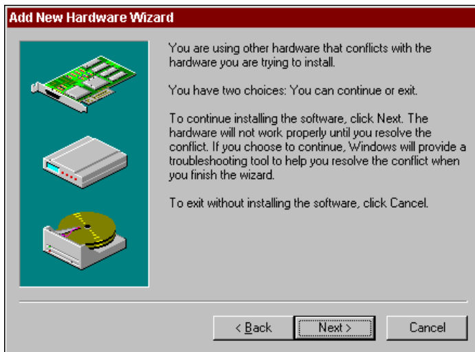
Figure 2-5. PC/104-GPIB Resources Not Assigned Successfully
